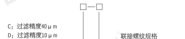
注:  $d_1 = G1\frac{1}{2}A$ , 过滤精度为 $40 \mu\text{m}$
